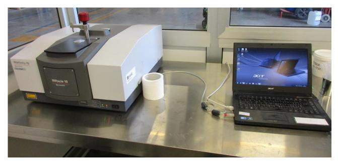
This is a Fourier Transform Infrared Spectrometer equipped with a an ATR (Attenuated Total Reflectance) device that permits us to analyze liquid and solid sapmples. This instrument has a signal to noise ratio (S/N) of 30.000/1 cm<sup>-1</sup> and it can cover a spectral range from 400 to 4000 cm<sup>-1</sup>.
