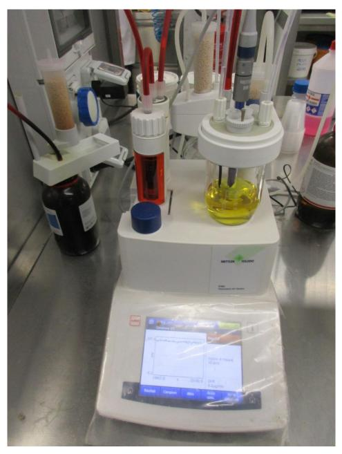
This is an automatic Karl Fischer Titrator that we use to determine the water content of polyether polyols used in the synthesis of polyurethane prepolymers. The amount of water must below 0.1% w/w, otherwise this could cause serious problems to the polymerization process.
